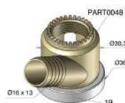
Base 7 M30 threaded base With vacuum Ø16 x 13 Internal diameter Ø26 Nylon or steel nose piece
